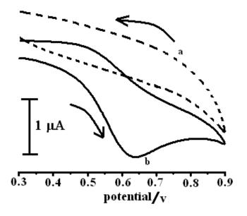
**Fig. 1.** Cyclic voltammogram of enzyme electrode in 0.1M phosphate buffer, pH 7.0 and 0.1 M KCl (a) without substrate (dashed line) (b) with 1 mM substrate (solid line)
