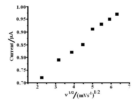
**Fig. 3.** The enzyme electrode response by varying squareroot of scan rate for 1 mM ASChCl in 0.1 M phosphate buffer (pH 7.0) and 0.1 M KCl
