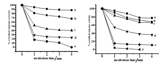
**Fig. 7.** Effect of incubation time on residual enzyme activity for various inhibitor concentrations in 0.1M phosphate buffer / KCl pH 7.0 (A) For Quinalphos (a) 20 ppb (b) 50 ppb (c) 200 ppb (d) 250 ppb (e) 300 ppb (B) For Malathion (a) 0.07 ppm (b) 0.1 ppm (c) 0.15 ppm (d) 0.40 ppm (e) 1.0 ppm (f) 1.3 ppm
