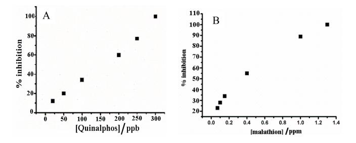
**Fig. 6.** Inhibition plots of (A) Quinalphos after 4 min incubation time (B) Malathion after 4 min incubation time in 0.1 M phosphate buffer (pH 7.0)/0.1 M KCl
