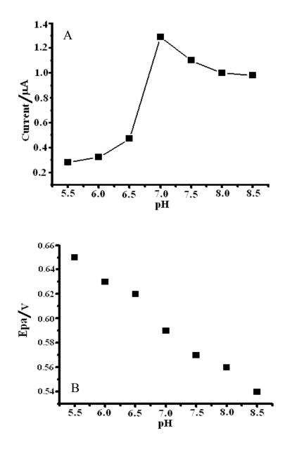
**Fig. 4.** (A) Effect of the pH on the enzyme electrode response (B) Plot of Ep<sub>a</sub> *vs.* pH to 1 mM ASChCl
