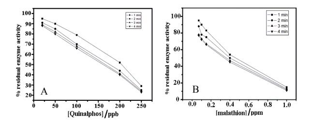
**Fig. 9.** The variation of residual enzyme activity with different inhibitor concentrations with respect to time in 0.1 M phosphate buffer / 0.1 M KCl, pH 7.0. (A) For quinalphos, (B) For malathion
