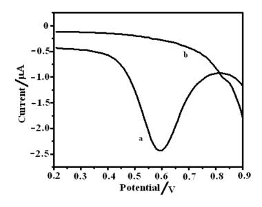
**Fig. 8.** Differential pulse voltammograms of (a) substrate alone (b) with 300 ppb of quinalphos/1.3 ppm of malathion pesticide solution
