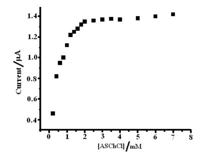
**Fig. 2.** Calibration graph for acetylthiocholine chloride obtained with AChE immobilized sensor in 0.1 M phosphate buffer / 0.1 M KCl at pH 7.0
